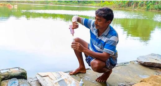
Water testing kit to monitor water quality parameters for adaptive measures to increase fish production in this climate changing scenario
